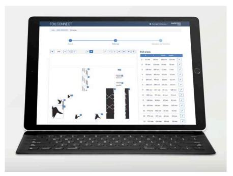
Based on a PDF file of stamping designs, the Kurz Foilconnect program calculates the optimal usage of hot stamping foils.
