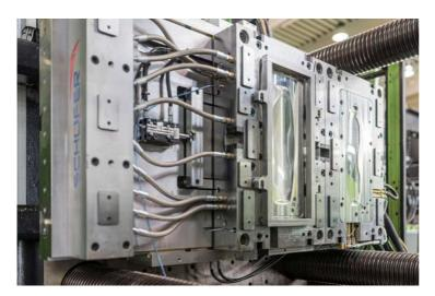
Injection mold in which injection molded parts are provided with an in-mold decorative design and PUR topcoat by means of Kurz's IMD PUR technology. (Photo: Kurz)
